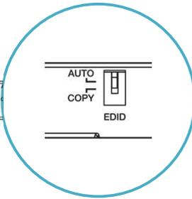
When copying EDID, connect your display device to Output-1. Recycle power every time settings are adjusted.
